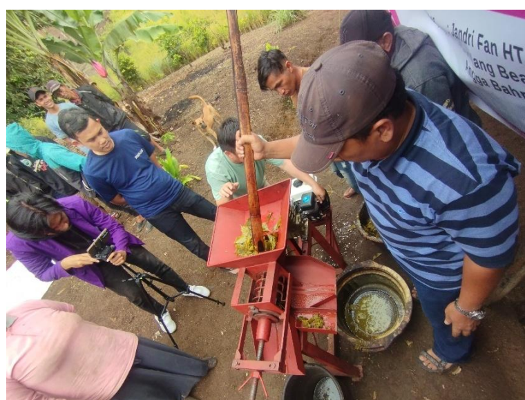
Figure 4. Gambir Processing using a Screw Press Machine
